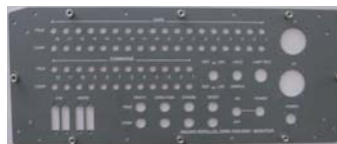
Wet painted aircraft test set panel
